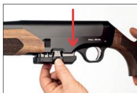
2. Unscrew the forend nut and push the forend forward while holding the receiver.
