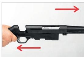
4. To remove the bolt carrier, separate the slide from the slide levers with a straight screwdriver. After that hold the bolt carrier and pull it all the way back.
