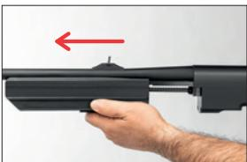
3. Hold the barrel group with one hand and hold the lower receiver with your other hand, at the same time. Remove the upper side from the lower receiver by pulling it forward..
