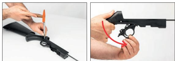
7. To disassemble the buttstock, push the recoil pad plunger pin and pull the recoil pad backwards. After removing the recoil pad, unscrew buttstock assembly screw with using special tool (5mm Allen Wrench Set) for it and separate them.
