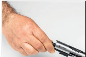
5. To remove the barrel from the upper receiver, unscrew the barrel assembly screw with 12mm wrench and separate them.
